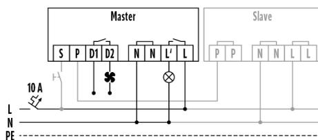
Standard operation with optional control via a closing button and use of max. ten slave devices to one master device.
